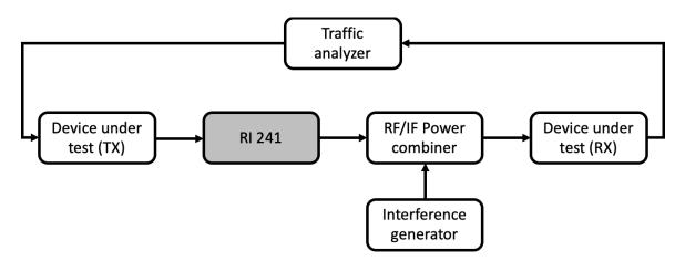
Receiver sensitivity measurements (carrier to noise characterization) is done by simply setting the wanted carrier to noise level (C/N<sub>0</sub> in dB) from the RI 241, while monitoring the traffic quality recorded by the traffic analyzer (e g Bit Error Rate, BER). Six different noise bandwidths are selectable and the C/N<sub>0</sub> can be set in 0.1 dB steps.
