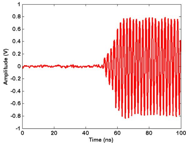
Figure 18a: Pulse Mod Rise Time,  $f_c = 500\text{MHz}$
