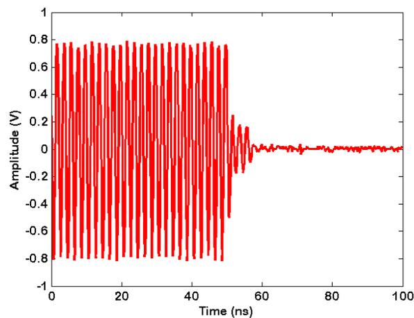
Figure 19a: Pulse Mod Fall Time,  $f_c = 500\text{MHz}$
