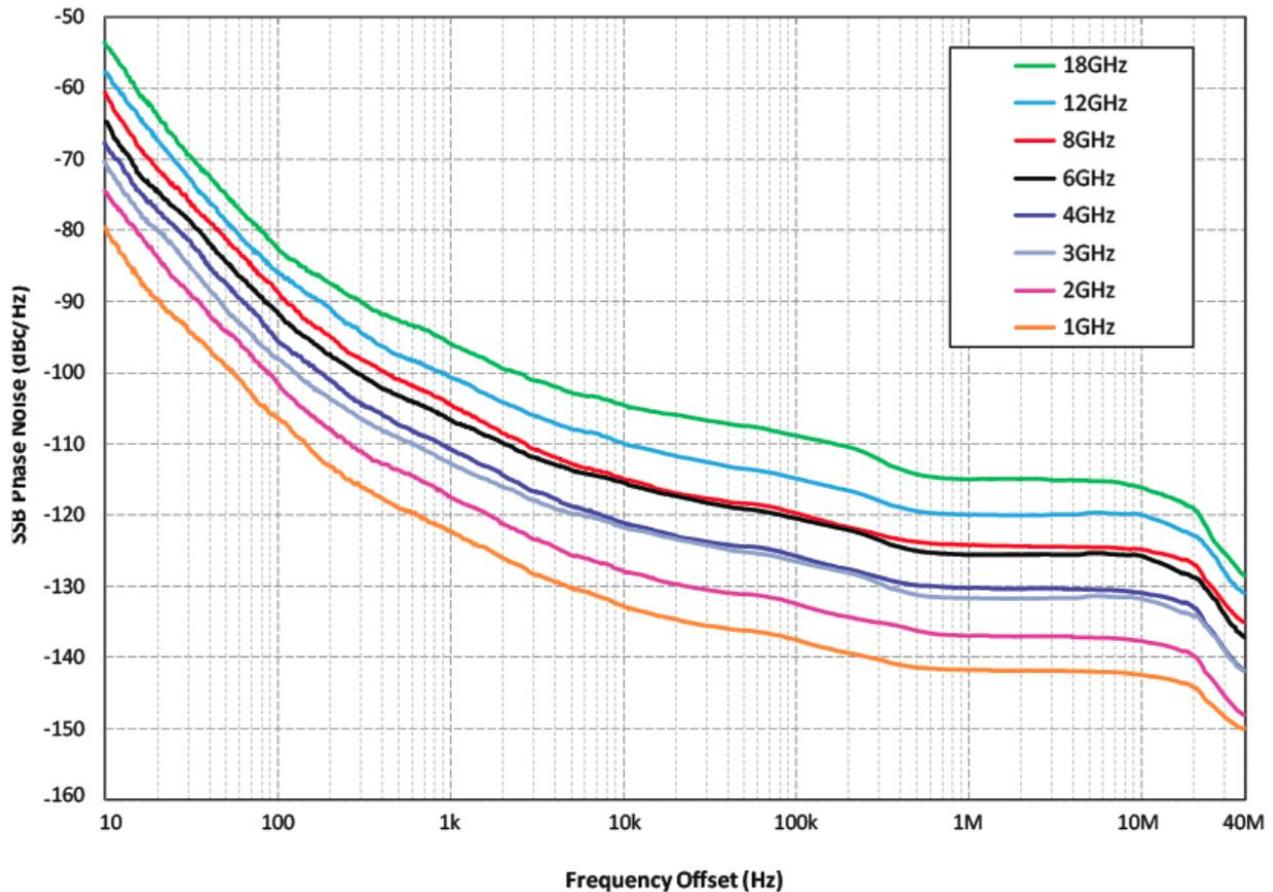
Figure 10: Phase Noise Performance (typical), P<sub>OUT</sub> Setting: +10dBm
