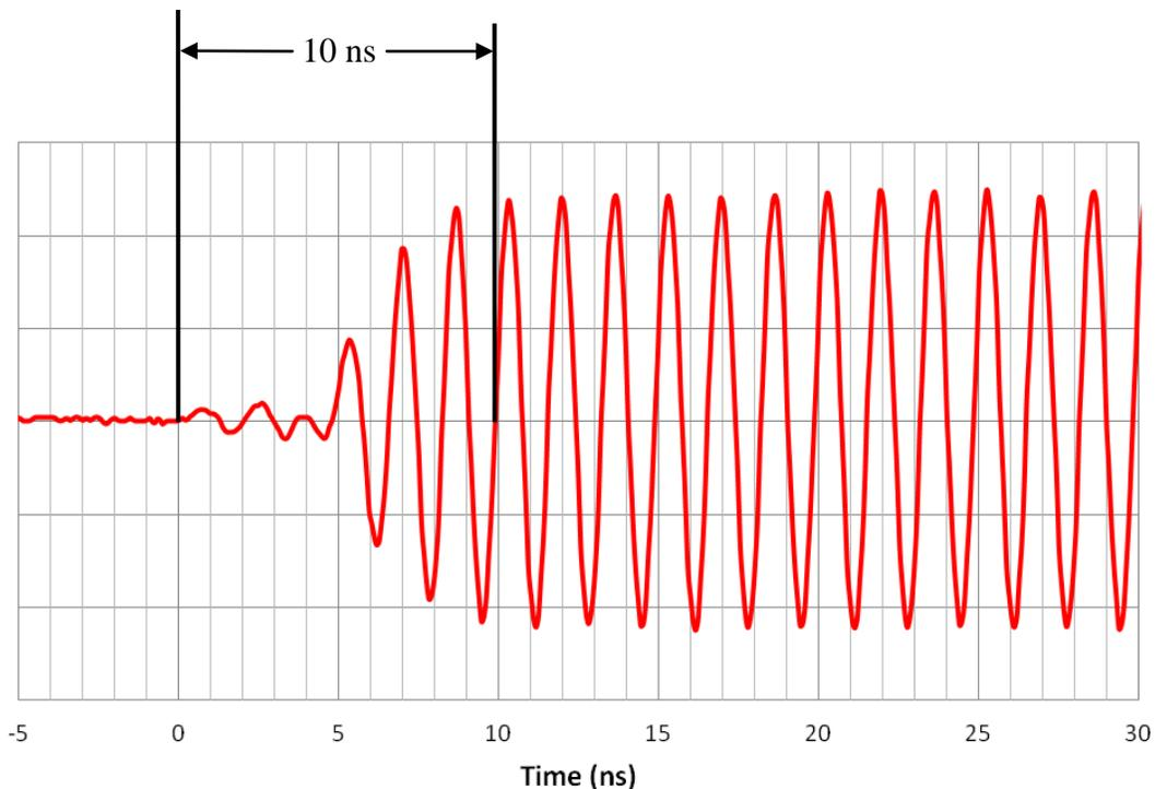
**Figure 20: External Pulse Modulation Rise Time (seconds)**
