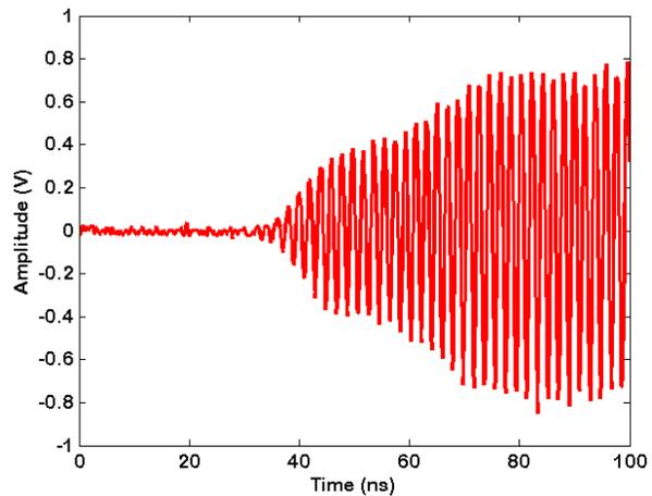
Figure 18b: Pulse Mod Rise Time,  $f_c = 530\text{MHz}$
