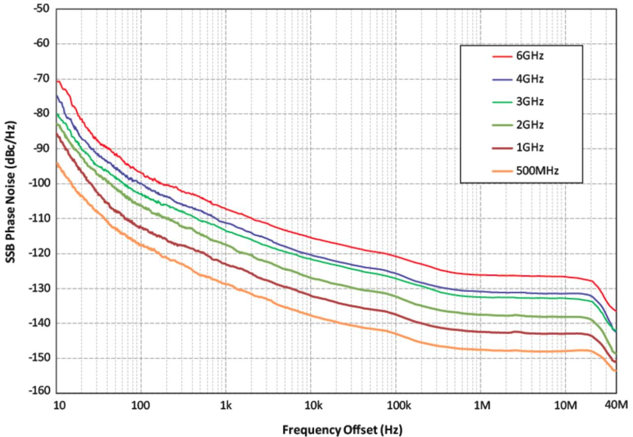
**FIGURE 3: Phase Noise Performance (typical), P<sub>OUT</sub> Setting: +10dBm**
