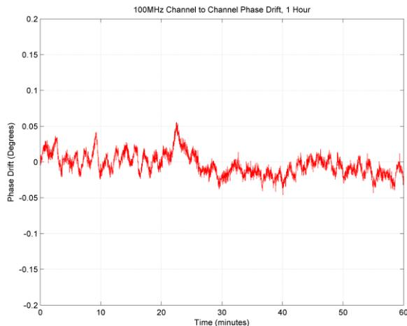
**Figure 21a: 100MHz Phase Drift (1hr, 20C)**
