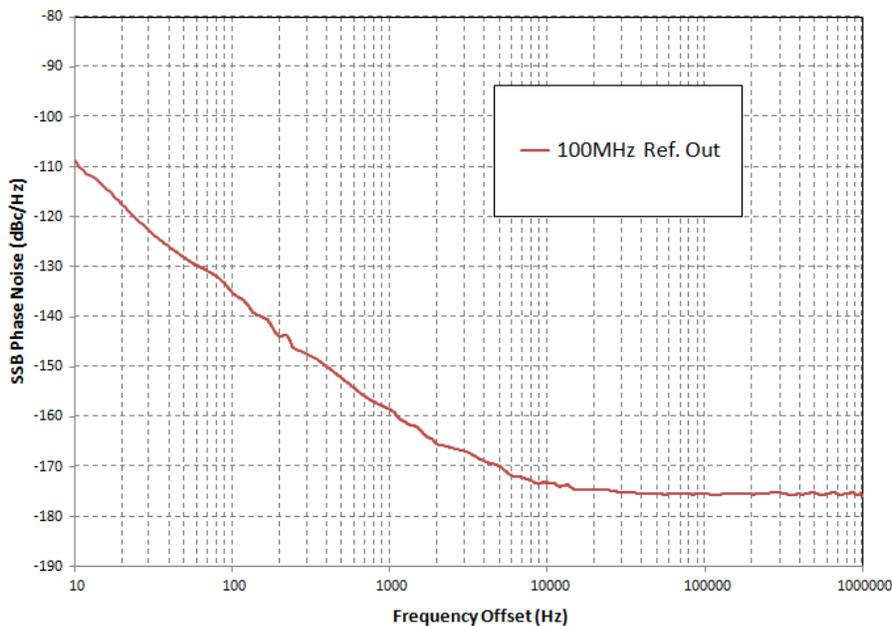
**Figure 16: 100MHz Reference Output SSB Phase Noise**
