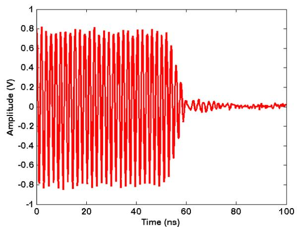
Figure 19b: Pulse Mod Fall Time,  $f_c = 530\text{MHz}$
