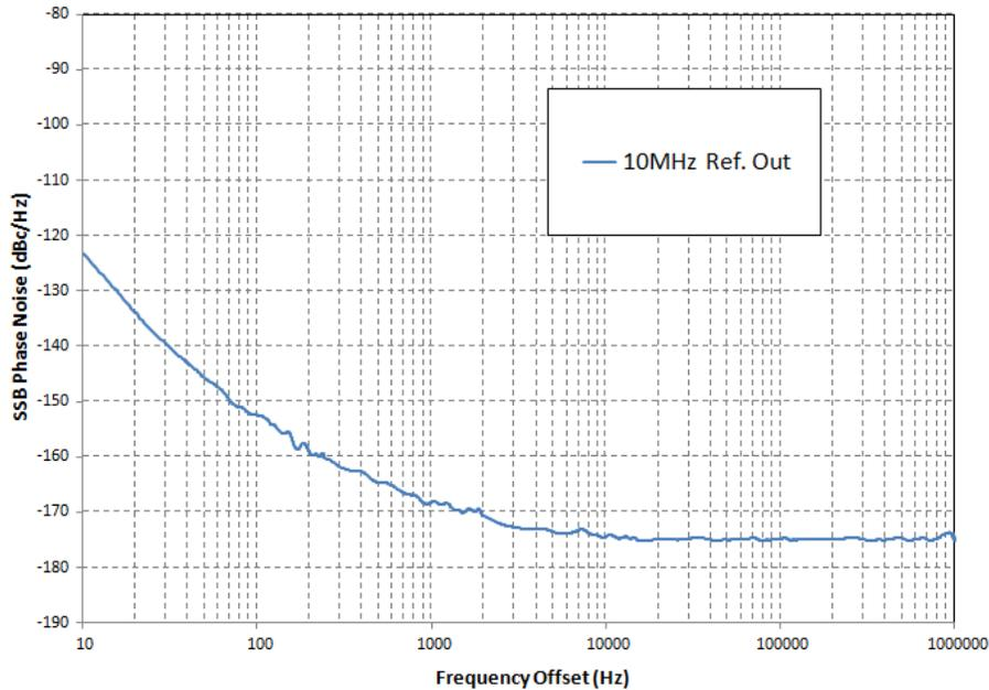
**Figure 15: 10MHz Reference Output SSB Phase Noise**
