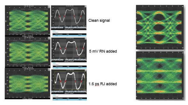
Figure 11: Adding impairments to a 26/53 GBd signal using the ML407PAM clock synthesizer
