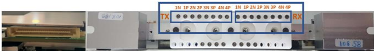
Figure 4: AT4039EML Pinout. Closest to the backplane connector is TX1N
