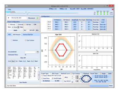
Figure 3: Single layout of Contour for one channel
